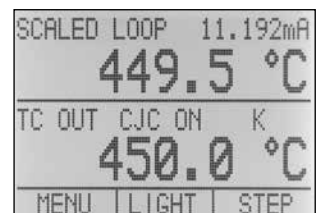
Online scaling, difference shown in the actual unit, saves calculation time and potential errors in the field
