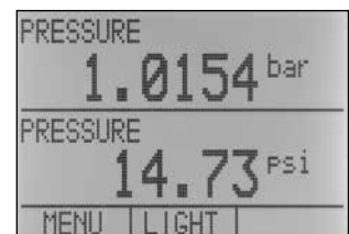
Dual pressure display measurements enable easy pressure conversion
