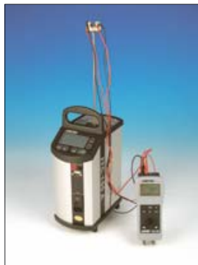
CSC200 as RTD input with an ITC
