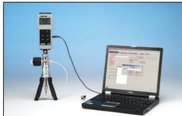
Set-up with JOFRA APC system B connected to a PC with JOFRACAL
